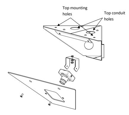
Figure 2 - Exploded View of Corner Camera
