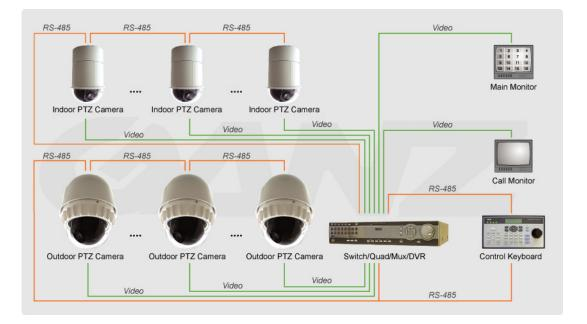
**NOTE:** The use of a repeater is recommended if the system network distance exceeds 1.2 km (4000 feet). In this case, placing the repeater at the centre of the network distance could help to maintain signals. Refer to the repeater user manual for detailed information.
