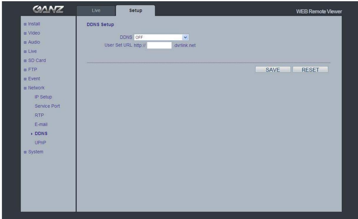
The GANZ Dynamic Domain Name Service (DDNS) can provide your GANZ product with its own name server address (URL), which can then be used to access it over the Internet. The product can be unregistered from the service at any time. To do this click Network > DDNS and turn the DDNS off.
