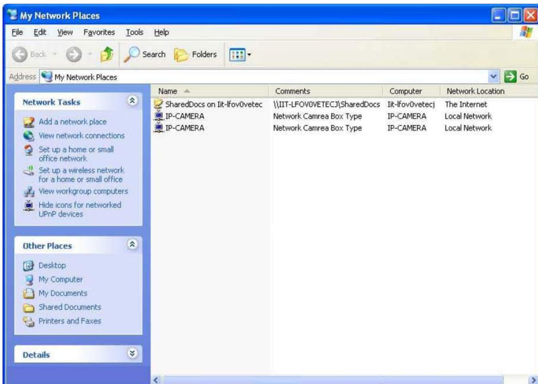
In order to be able to detect the camera automatically, you must enable the UPnP function on both the camera and on your PC.
