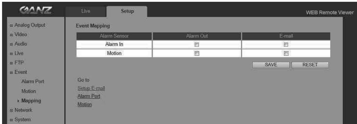
It is possible to define conditions that would cause the camera to respond with certain actions. A triggered event happens as a result of a trigger, which could be motion detection or an external alarm input.
