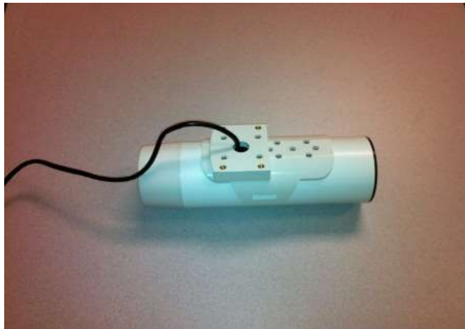
Camera with Base mount and Standard 4-Hole mount
