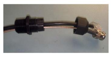
4. Tighten the gland nut onto the gland housing. Leave about 5 inches of cable sticking out of the gland housing
